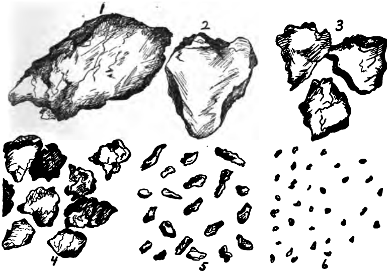
FIG. 1. Medium sand \times 150 . FIG. 2. Fine sand \times 150 . FIG. 3. Very fine sand \times 150 . FIG. 4. Silt \times 325 . FIG. 5. Fine silt \times 325 . FIG. 6. Clay \times 325 .
